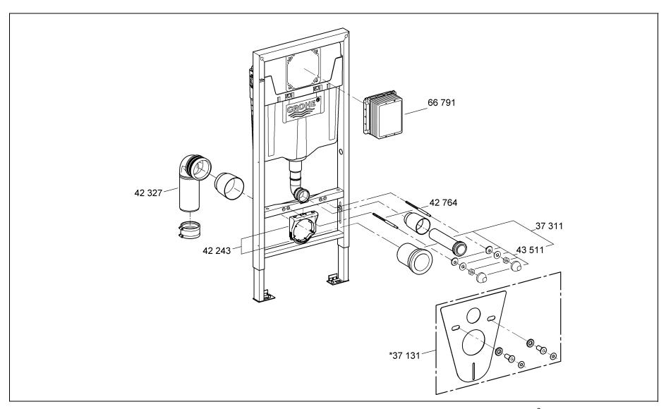
The tank and carrier are designed to fit within a 2"  $\times$  6" wood frame (or equal) construction. The studs must be placed 19  $^3/_4$ " apart at the location where the unit will be positioned prior to installation into the wall. The carrier legs must be adjusted for the finished rim height of the water closet bowl. The dimensions may be taken from the bowl or from the specification sheet. Be sure to allow for finished floor covering.
