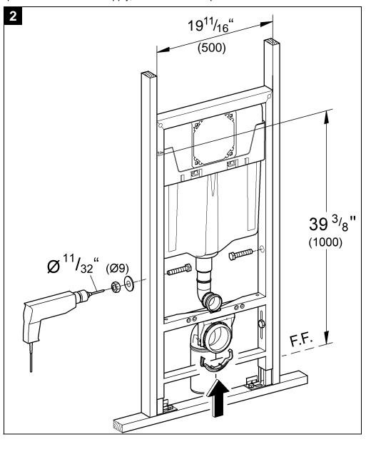
**STEP 4:** Install 3" DWV waste pipe through floor and connect to waste line (i.e. PVC, copper, cast iron).
