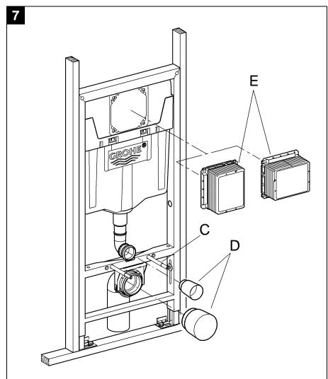
**STEP 8:** Install two  $^{1}/_{2}$ " x 6" fixture support rods with plastic sleeves (C), the pipe caps (D) and mud guard (E) are mounted for protection during wall surface construction, see fig. [6].
