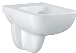
39809000 BauEdge WC wall hung, rimless, for concealed cistern, horizontal outlet, flush volume 3/5 l, washdown, compatible with seat and cover (seat sold separately)
