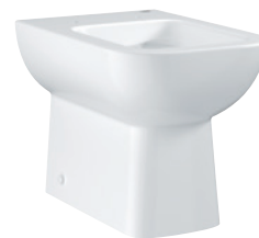
39810000 BauEdge floorstanding WC pan Washdown back-to-wall rimless Horizontal outlet, 5/3 l flush. For concealed cistern, (seat and concealed cistern sold separately)
