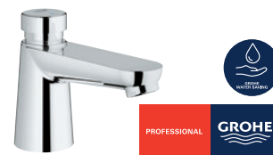
36265000 £128.63 Euroeco Cosmo T self-closing pillar basin mixer GROHE Water Saving mousseur 5.7 l/min Three adjustable flow times: Short - medium - long (factory setting: short), approx. 7, 15, 30 sec (pressure dependent)
