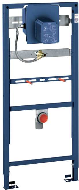
Rapid SL Element for urinal for flush plate actuation, 1.13 m installation height. GROHE no.: 38 786 001
