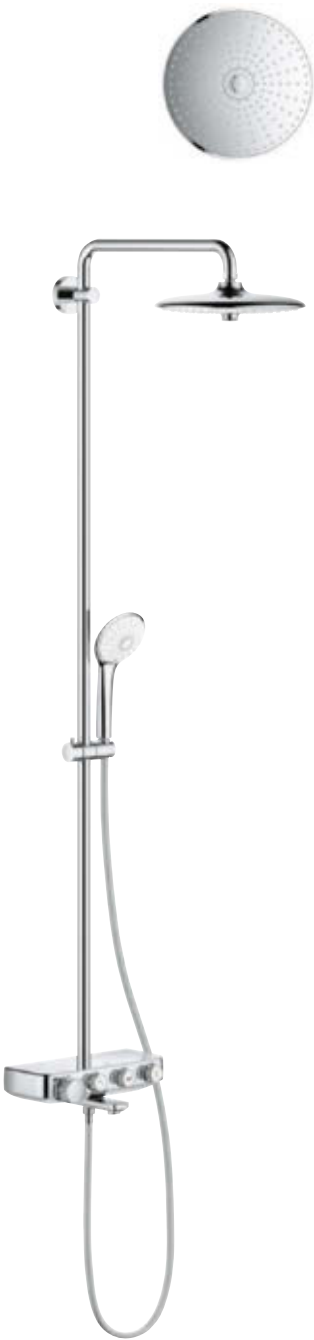
26 608 000 / 26 510 000 Euphoria SmartControl 260 Bath/Shower System with bath thermostat for wall mounting consisting of: Head Shower Euphoria 260 (26 455) 3 spray patterns: Rain, SmartRain, Jet with ball joint, Hand Shower Euphoria 110 Massage, 3 spray patterns: Rain, SmartRain, Massage spray plate white (27 221 001) Silverflex shower hose 1750 mm (28 388) Rail length 997 mm (26 608 000) Rail length 1452 mm (26 510 000)
