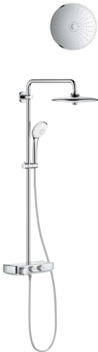
26 509 000 Euphoria SmartControl 260 Shower System with thermostat for wall mounting consisting of: Head Shower Euphoria 260 (26 455) 3 spray patterns: Rain, SmartRain, Jet with ball joint, Hand Shower Euphoria 110 Massage, 3 spray patterns: Rain, SmartRain, Massage spray plate white (27 221 001) Silverflex shower hose 1750 mm (28 388)
