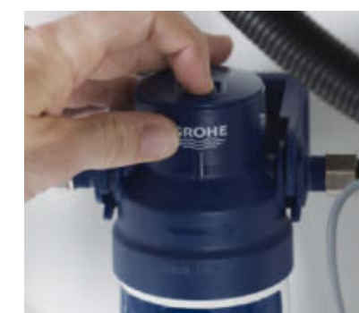
Set-up filter head by-pass and capacity counter according to the water hardness.
