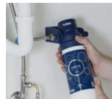
Attach filter holder to the cabinet and screw filter into filter head. Then connect the filter to the cold water supply.
