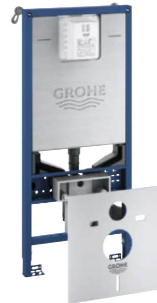
39 598 000 Rapid SLX 3in1 WC 6 | 1.13 m with wall brackets and noise protection Rapid SLX Element for WC, 1.13 m installation height with flushing cistern GD2, with electric socket, including flow manager, easy access and fully insulated against condensation. With wall brackets and noise protection.
