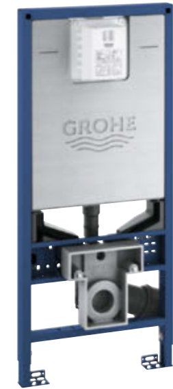
39 601 00D Rapid SLX WC 3-6 | 1.13 m, SASO Rapid SLX Element for WC, 1.13 m installation height with flushing cistern GD2, with electric socket, including flow manager, easy access. Specifically for Saudi Arabia with different settings.
