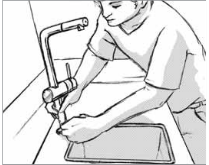
2. You can assemble the faucet and connections in the sink.
