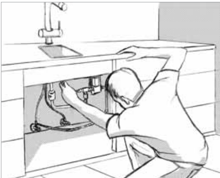
3. Connect the fitting to your water connections as usual. Now connect the EasyTouch technology battery-operated control unit between fittings and cold-water connection. Done.
