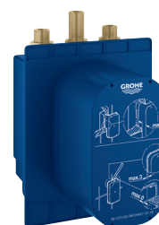
36 416 001 Concealed body for shower with transformer 100 – 240 V AC and integrated pre-adjustable thermostatic mixer suitable for infra-red set 36 415 000 and 36 463 000
