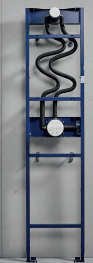
On the wall installation with wall mounting set sold separately 112-172 mm (installation depth to front of frame) Perfectly fits stud wall installation > 67 mm (depth up to front side of frame)
