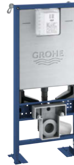
39 599 000 Rapid SLX WC 3-6 | 1.13 m F with heavy load feet Rapid SLX Element for WC, 1.13 m installation height with flushing cistern GD2, with electric socket, including flow manager, easy access and fully insulated against condensation. With heavy load feet.
