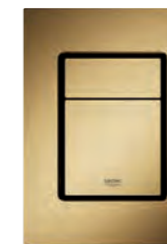
38 732 GN0 Skate Cosmopolitan Flush Plate Dual Flush or start & stop actuation for pneumatic drop valve AV1 for vertical and horizontal installation GROHE Long-Life Shine durable sparkling sheen GROHE Water Saving - Less water, perfect flow for combination with Rapid SL 1.13 m with GD 2 cistern for use with Rapid SLX please order shaft 66 791 000 (sold separately) 197 x 156mm
