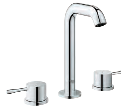
20 596 001 Basin set with separate concealed body Pressure-proof flexible connection hoses between spout and side valves union nut 1/2" X 10.5mm WELS 5 Star, 6 ltrs/ min
