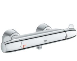
34 667 000 Grotherm Special Thermostatic shower mixer, wall-mounted with pre-adjustable safety stop between 35 °C and 41 °C
