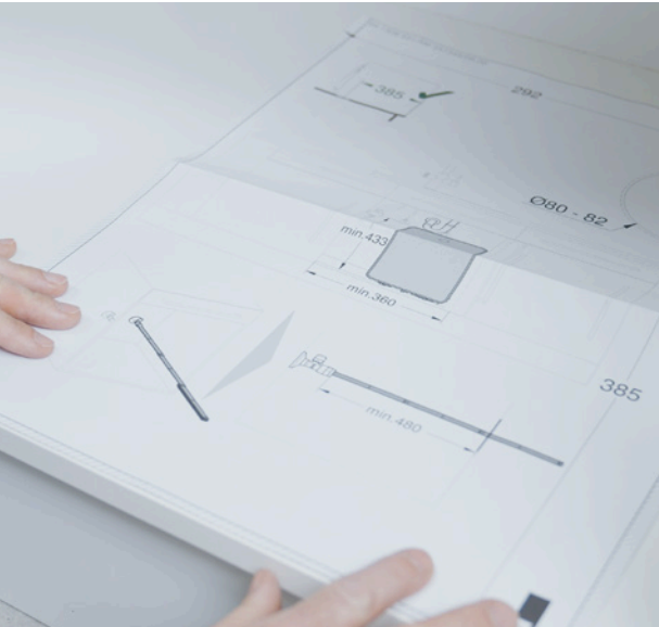
02 CORRECTLY POSITION THE INSTALLATION TEMPLATE IN THE CABINET
