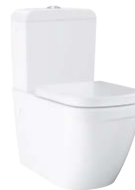
39 462 000 / 00H* WC closed coupled combination: WC, rimless, Triple Vortex, wash down, universal outlet (39 338 000 / 00H) Cistern with bottom inlet (39 332 000) Seat & cover soft close (39 330 001)
