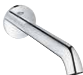
13 392 001 Bath spout wall mounted projection 220mm female thread 1/2"
